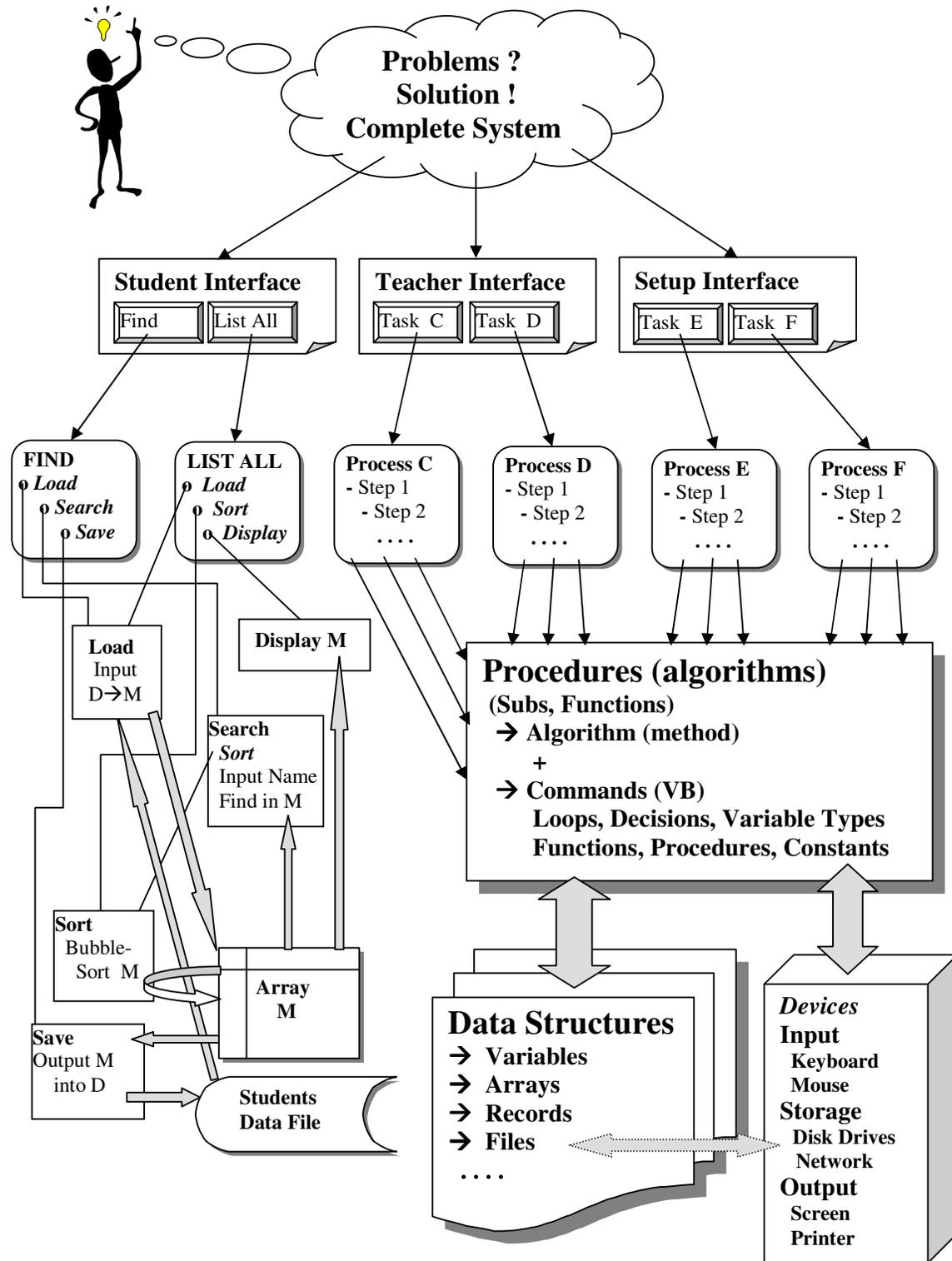
Normally the **data-structures** do not appear on the same diagram with the **procedures**. This was done here to illustrate the relationship between **algorithms** and **data-structures**.
