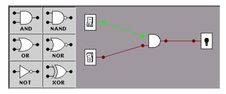
This circuit contains a single AND gate. It represents a **burglar alarm.** The top switch turns the alarm on and off. The bottom switch represents a sensor in the door, which produces a signal when the door is opened. The light represents the alarm signal, which goes on if the door opens when the alarm is active.
