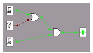
The circuit above represents a burglar alarm. One of the switches turns the alarm on and off. The other two switches represent sensors: one sensor on a door, the other sensor on a window.
